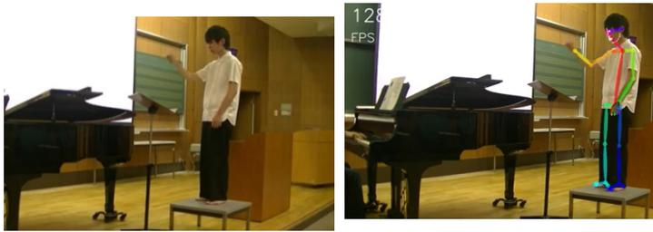
Fig. 7 Estimated joint parts from 2-D motion pictures
