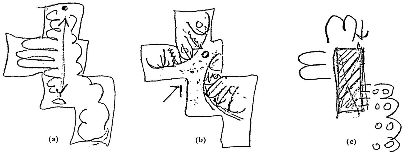
**Figure 7.** *Alternative Library Plans Using Different Entry Points: (a). Long Entry Hall Between Reading Rooms and Stacks, (b). Open Plan With Interior Court, and (c). Library Elements Surrounding Atrium*
